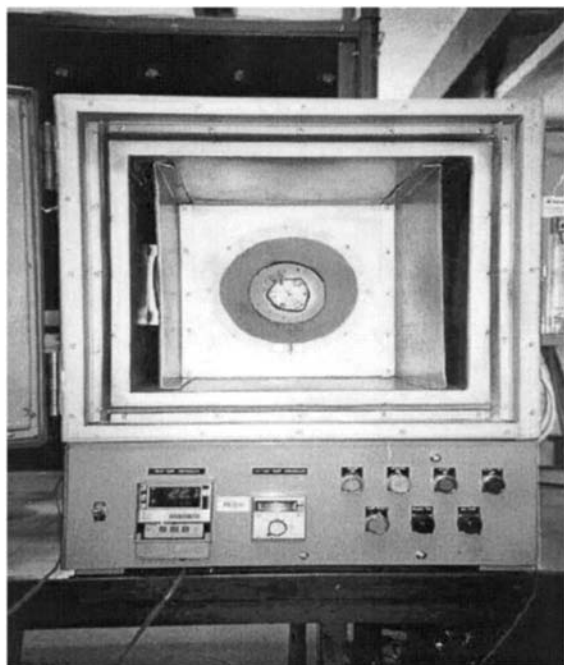
Fig. 1. Interior view of the adiabatic oven.
